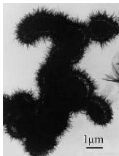
Figure 6. TEM pattern of the products obtained at 0 °C (aging for 10 h).
